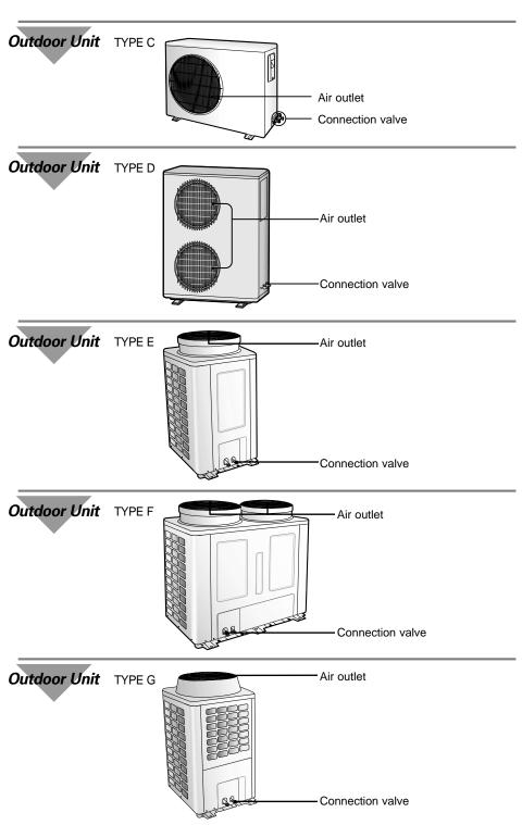
Mote If the heat exchanger in the outdoor unit gets dusty, cooling efficiency may fall. So clean the heat exchanger with water when it becomes dirty. However, be careful when you wash the surface of the heat exchanger because it is very sharp.
